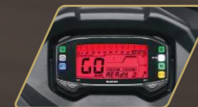
Smart digital Instrumentation with Gear position and RPM indicator
